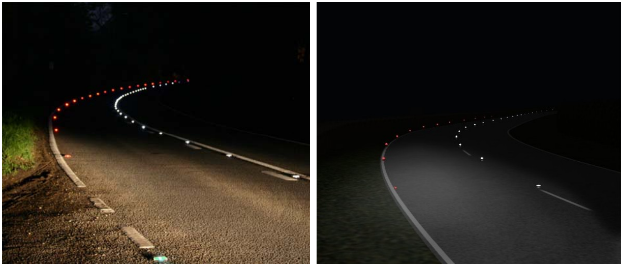
Figure 2.1 Real photograph (left panel) and screenshot from the simulated road environment (right panel) each showing centre-line white studs and nearside edge red studs
